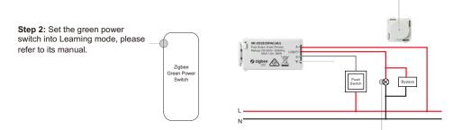
Step 3: Connected light will flash twice to indicate successful learning. Then the switch can control the device.
