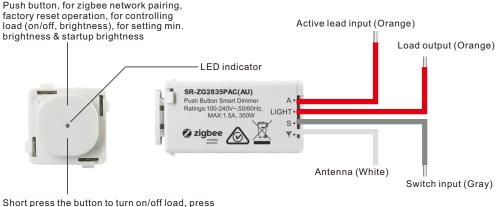
Short press the button to turn on/off load, press and hold to dim up/down the load between the range 1%~100%
