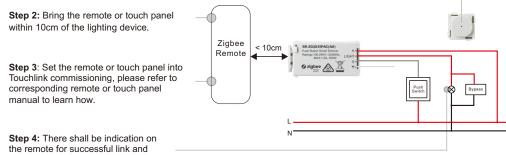
the remote for successful link and connected light will flash twice. Note: 1) Directly TouchLink (both not added to a ZigBee network), each device can link with 1 remote.
