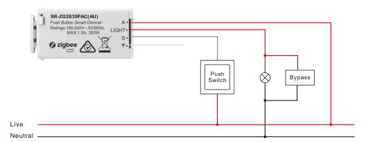
**NOTE:** Switch connected to the switch wire activates the basic functionality of the dimmer (short press to turn the light on/off, hold to dim up or dim down).
